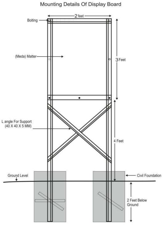
**B** Mounting Details Of Display Board
